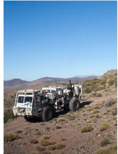
Vibroseis truck for conducting seismic surveys in Mendoza
