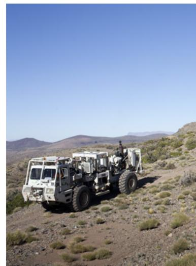
Thumper truck for conducting seismic surveys in Mendoza
